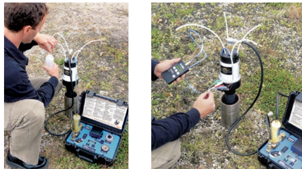
Figure 7-1 Testing Pumps and Transducers
