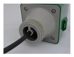
3 - Slide the microphone tubing into the spout and connect the Well Watch to the spout with the plastic ring nut.
