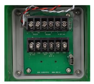
6 - Attach signal wiring.
