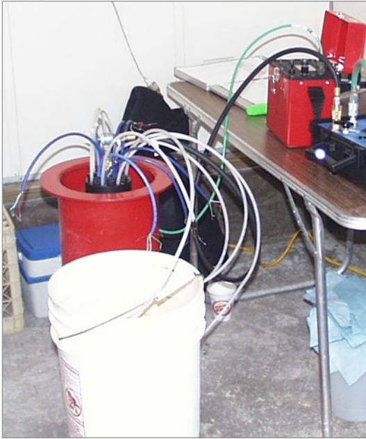
Four Waterloo Systems were installed to monitor a chlorinated compound release. Systems were installed at depths ranging from 131 m – 229 m (430 ft – 750 ft), with most monitoring 7 zones. The Ports were constructed with both Double Valve Pumps and Vibrating Wire Transducers.
