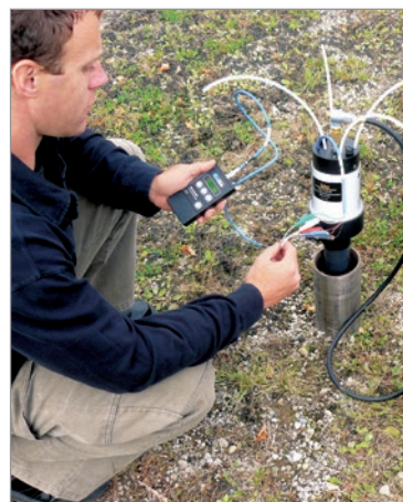
Collecting a sample from a dedicated DVP and taking pressure measurements with Model 404 Geokon Vibrating Wire Readout (above).
