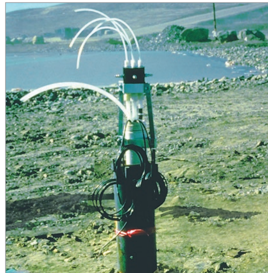
Landfill site over fractured granite, monitored with five Waterloo Systems. Each System comprised of dedicated Double Valve Pumps and Pressure Transducers in 4-6 intervals to depths of 84 m (275 ft). The Multi-Purge Manifold allowed the monitoring of 21 zones to be completed in less than 2 days.
